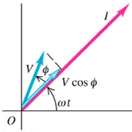
$$\hat{V} = V_0 e^{i(\Omega t + \Phi)}$$
