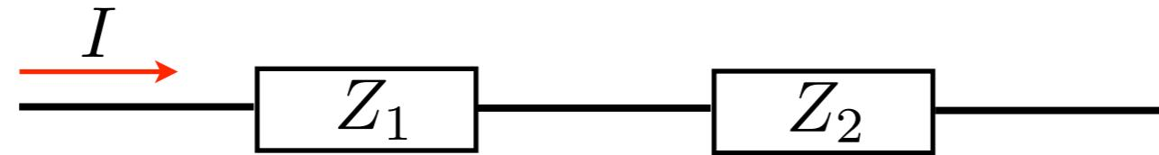
$$V = V_1 + V_2 = Z_1 I + Z_2 I = (Z_1 + Z_2)I$$
